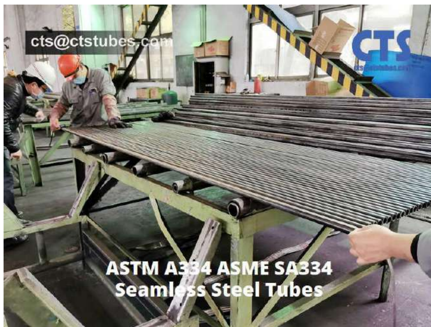
A334 GR.6 Seamless Tubes length inspection
