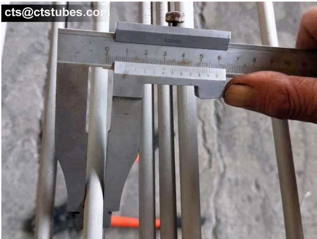
TP321 OD.10MM INSPECTION
