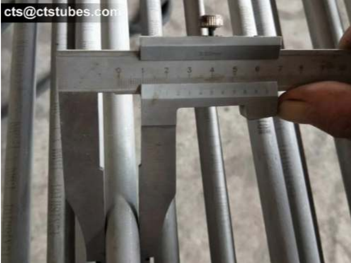
TP321 OD.15MM INSPECTION
