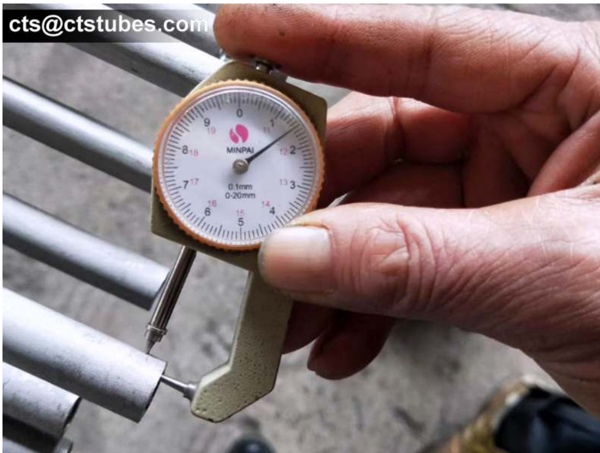
TP321 THICKNESS 1.5MM INSPECTION
