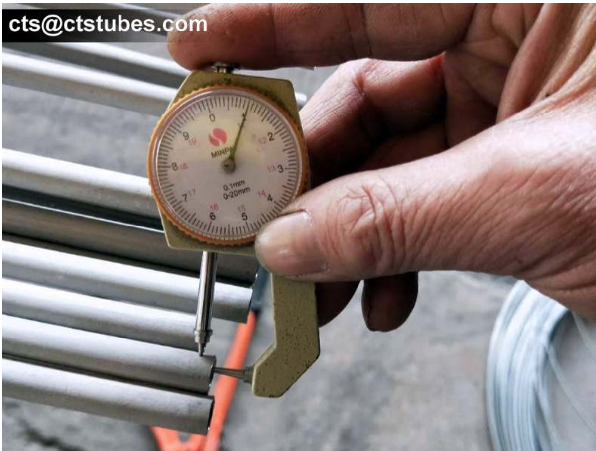
TP321 THICKNESS 1MM INSPECTION
